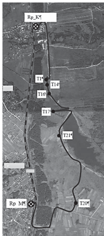
Fig. 2. Scheme of geometric spirit leveling of 2 class
